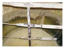
Liquid feed tanks must be cleaned on the inside to remove old feed, but it is not recommended to clean and disinfect the entire liquid feed system unless the liquid feed is of poor quality.
