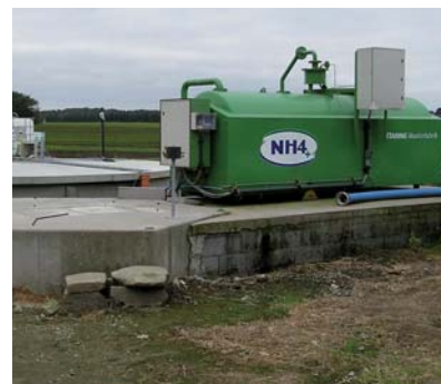
Behind the acidification system, the process tank can be seen and on top of that is a pallet tank containing a 30% hydrogen peroxide solution.
