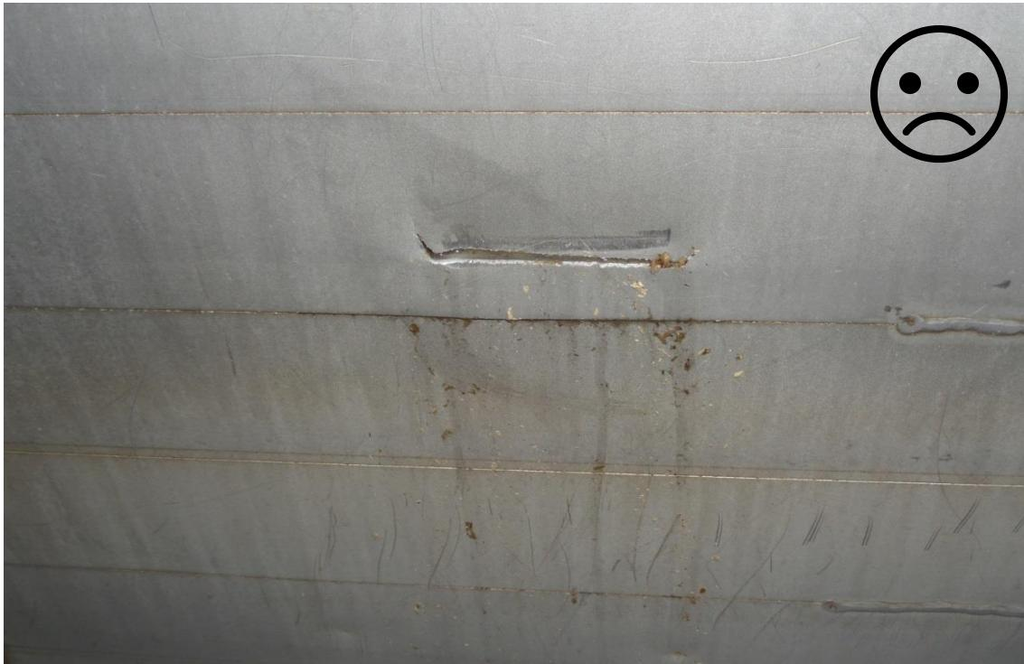
Figur 12. Skade/revne i vognsiden – AFVIST / Damage/crack in side of truck – REJECTED.
