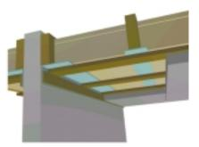
It is important to pass the section partition up through the mineral wool to prevent air from passing between sections. The membrane must lie on the lagging up against the mineral wool to prevent condensation.
