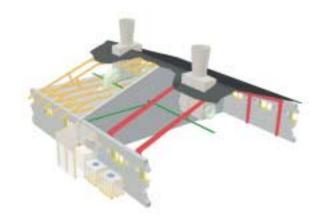
The system for chemical purification of the air is constructed with a central dosing and control unit from which the sulphuric acid solution is pumped to the exhaust pipes and is returned for collection.
