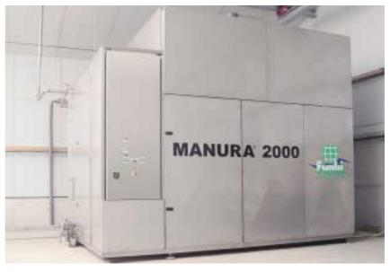
The Funki MANURA Compact belongs to the high-technological group. The slurry is separated into concentrated nutrients and "pure" water.
