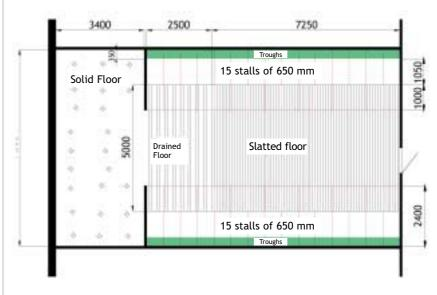
An example of a T-pen with continuous solid and drained floor.
