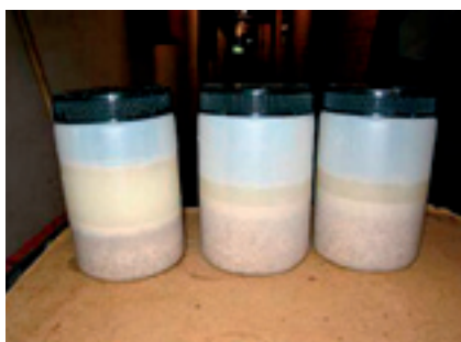
Collecting feed samples from different valves and comparing the sediment is an easy and quick way for checking feeding in systems with no residue.
