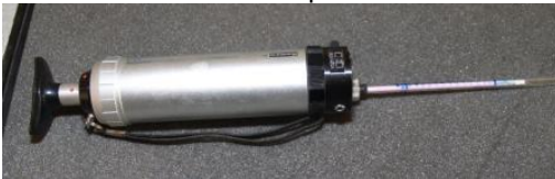
Pump and pipe for measuring ammonia
