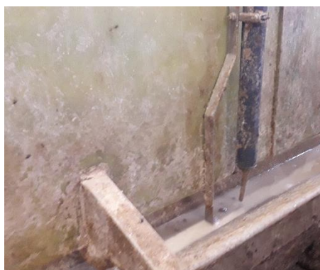
Sensor for feeding time control, mounted in the trough. Check sensors at valves with 0-values.
