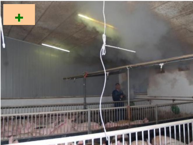
1. Smoke is used to check air flow
