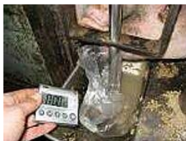
Check of water output in a feeder
