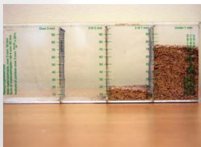
The feed must be ground finely to ensure a good feed conversion ratio.
