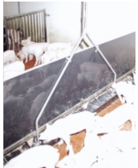
Baby-Feeder from W. Domino A/S can feed fresh liquid feed many times a day, in a long trough, for instance.
