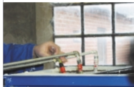
The liquid mineral pre-mixes were sprayed onto the feed while in the dry mixer.
