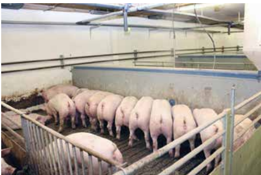
The dry feeding wall consists of a flex auger mounted on a pipe at the pen partition above the trough. Downpipes are installed for every 33 cm trough. The flex auger fills the pipe, which has two positions: one for filling and one for releasing feed through the downpipes. Flex auger and pipe are operated by a servo-motor.
