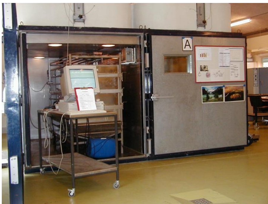
Figure 20.36. Physical activity may be recorded by a photo cell (visible left to the monitor). Infrared sensors were also recording the physical activity of the animals in the respiration chambers to record graded signals. Note that the door is only open to show the experimental setup, whereas the door had to be tightly closed during respiration trials (Photo: Henry Jørgensen).
