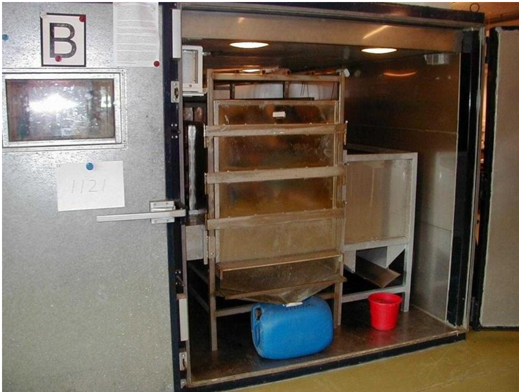
Figure 20.31. Collection of faeces is performed from the shelf below the animal, whereas urine from suckling piglets and the lactating sow is collected in the red and blue bucket, respectively (Photo: Peter Kappel Theil).
