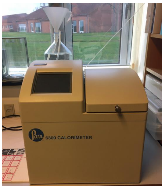
Figure 20.8. Parr 6300 Calorimeter, ISO-9831 [24]. (Photo: Henry Jørgensen).
